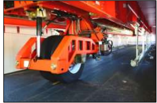
The weighted wheel assembly is on the underside of the heavy vehicle simulator (VDOT photo).
