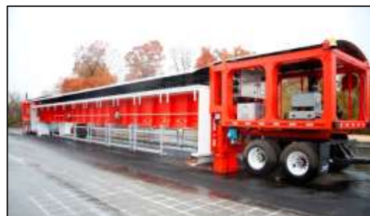
This heavy vehicle simulator is the technological heart of VDOT's new 'accelerated pavement testing' program (VTTI photo).
